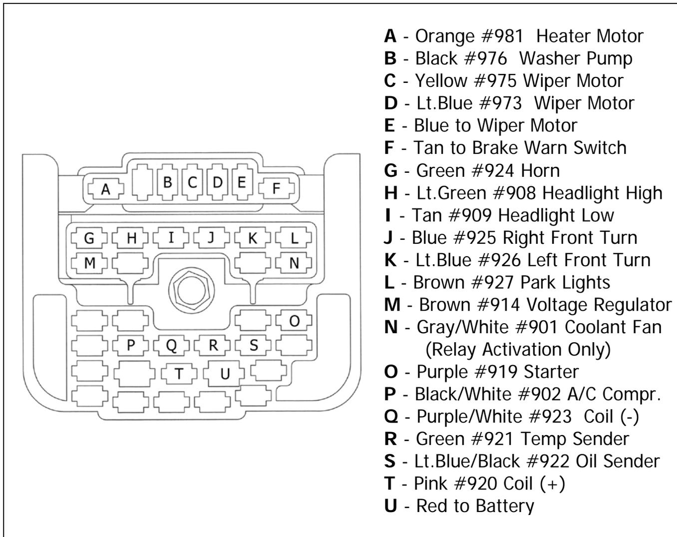
**Illustration 2** Engine Harness Firewall Connector Style #2
