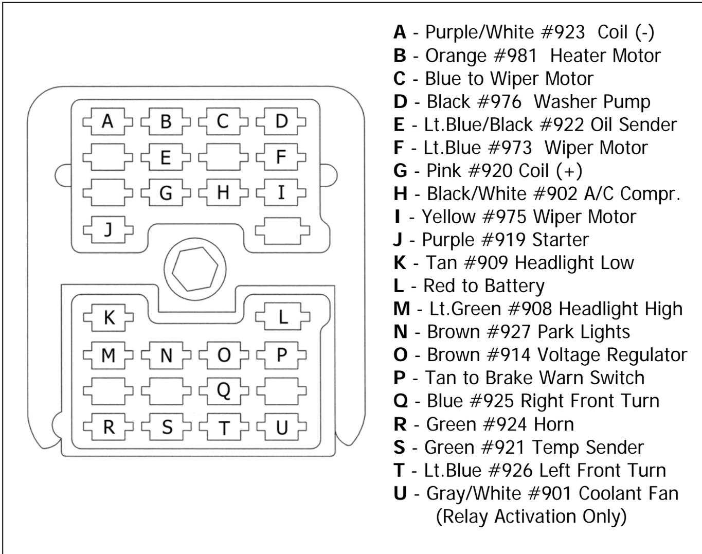
**Illustration 1** Engine Harness Firewall Connector Style #1
